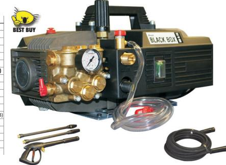
Safety classification Class A 1,800 (124 bar) Pump pressure psi Max rated pressure psi 2,175 (140 bar) EWP with turbo 3,400 psi Flow lpm 8 Single phase (240V) Motor Phase 2.6kW Power kW 1450 Pump speed rpm Triplex pump Pump type 035 Nozzle size Accessories -Hose 8m wire braid AL13 (M4021108008) Gun Vario Lance Turbo Lance M4048000038 Weight 30 kg Boxed dimensions LxWxH (mm) 390 x 240 x 230
