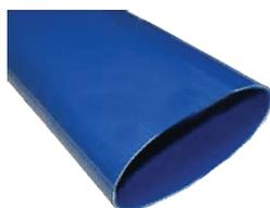
**Applications:** Lightweight layflat hose for potable water and other liquid foods. The construction of integrated tube and cover offers abrasion resistance five times higher than PVC. Also resistant to many acids, alkalis and other chemicals, and is UV and ozone resistant.
